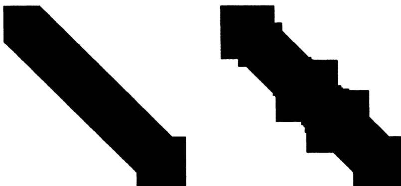
FIG. 6. Structure of factored matrix for version D and LAPACK algorithms.
